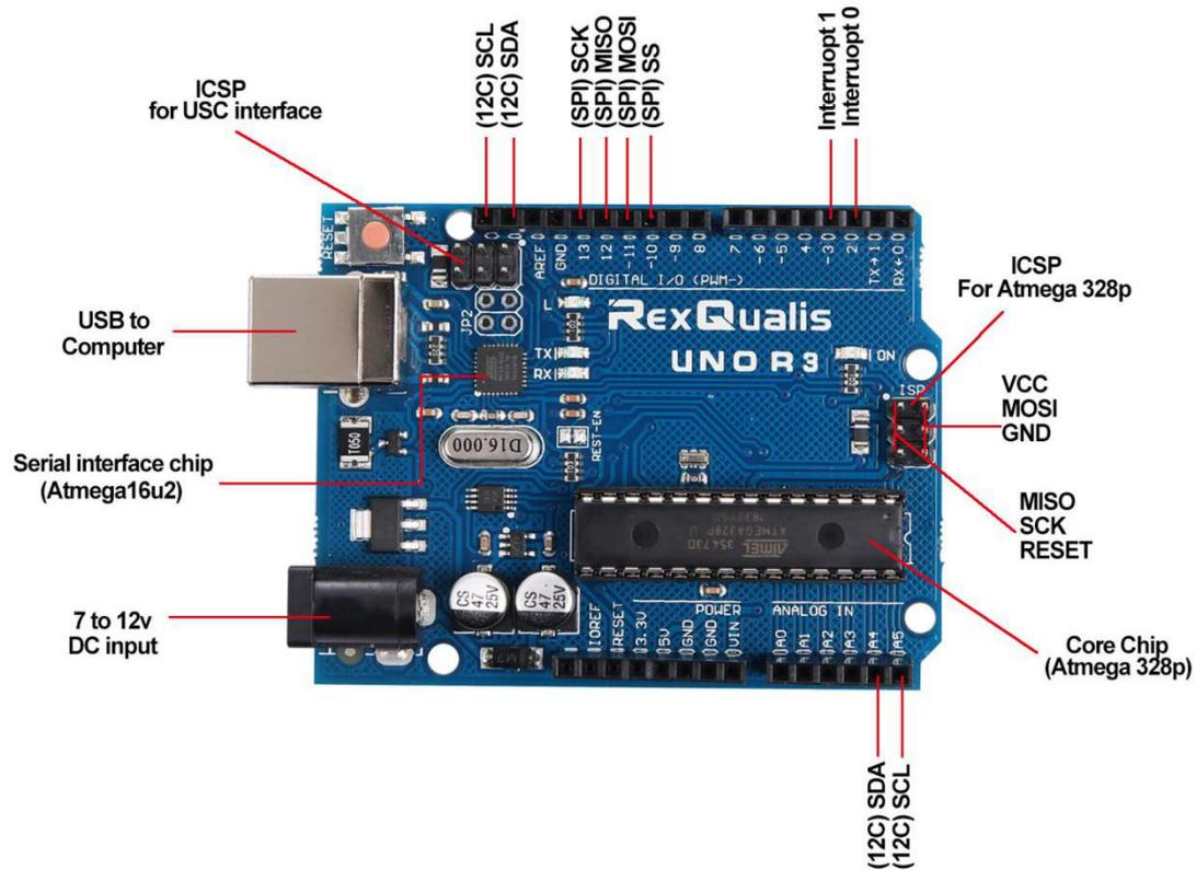
The top row of the Arduino has 14 digital pins, labeled 0-13. These pins can act as either inputs or outputs. You can connect them to your circuits to turn them on or off.
