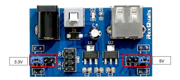
The left and right voltage output can be configured independently. To select the output voltage, move jumper to the corresponding pins.
