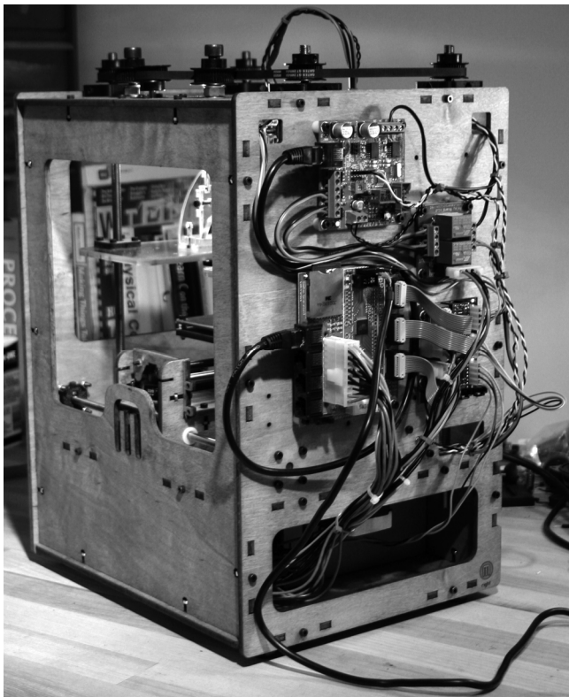
Figure 1-5. MakerBot CupCake 3D printer with Arduino-compatible electronics
