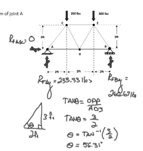
3) Calculate the force in member AC. Determine whether it is in tension or compression.
