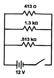
6) Total Voltage – Stay the same; Total Current – Decrease; Total Resistance – Decrease; Voltage drop at 0.513 Ohm resistor – Stay the same; Current at 1.3 Ohm resistor – Stay the same
